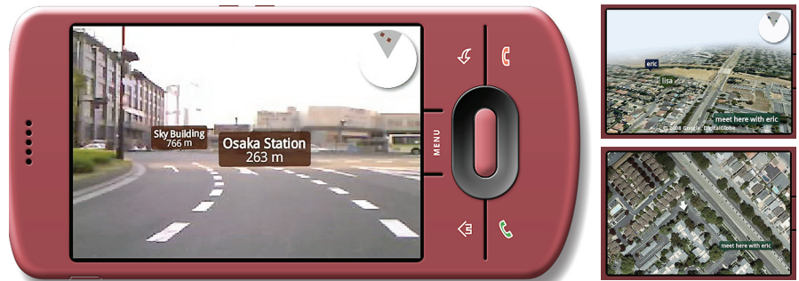
Enkin, a 3D navigation system built for Google's Android, provides a live mode via a video feed (left), a landscape mode (top right), and a map mode.
